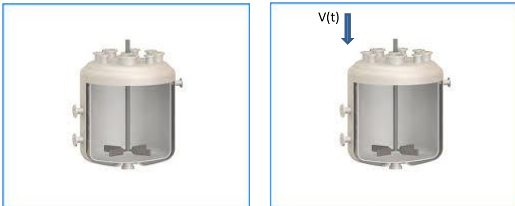
Gambar 24. Contoh reaktor (a) batch reaktor (b) semi batch reaktor
