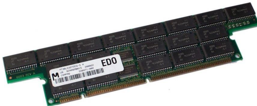
Gambar 2. 7 EDORAM (Extended Data Out Random Access Memory)
