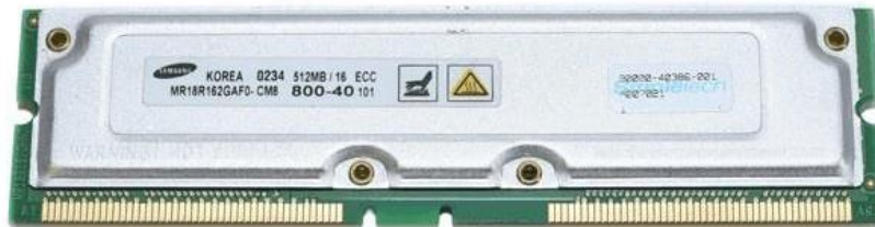
Gambar 2. 5 RDRAM ( Rambus Dynamic Random Access Memory )
