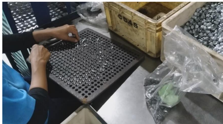
Gambar 4.6 Perakitan Valve Chamber
