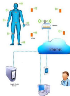
Gambar 2.3 Healthcare Monitoring System berdasarkan IoT
