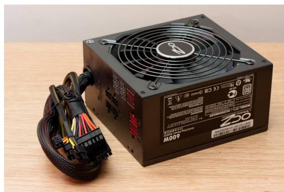
Gambar 2.10. Power Supply Jenis ATX
